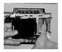
4. Mount the HDD: place the HDD in the slots on the bracket, then push the handle against the HDD to lock it in place.
